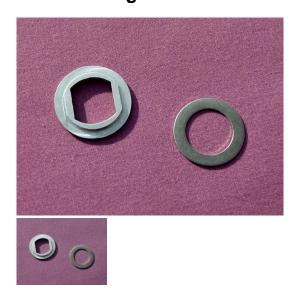
Faithful Fabrication of a Mills Vending Machine Lock Adapter
